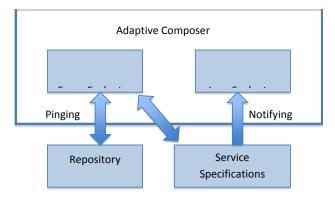
Figure 3 : Architecture of the Adaptive Service Composer or Composing Agent
