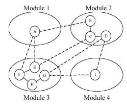
$\label{eq:figure 2} FIGURE~2$  COHESION AND COUPLING OF SOFTWARE MODULES IN CBSS
